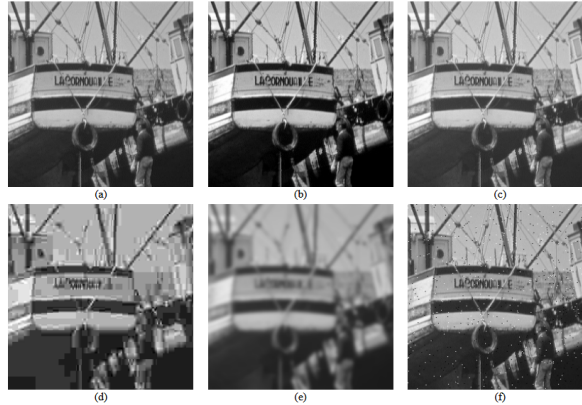
Figure 3.34: Comparison of “Boat” images with different types of distortions, all with MSE = 210 . (a) Original image (8 bits/pixel; cropped from 512 \times 512 to 256 \times 256 for visibility); (b) Contrast stretched image, MSSIM = 0.9168 ; (c) Mean-shifted image, MSSIM = 0.9900 ; (d) JPEG compressed image, MSSIM = 0.6949 ; (e) Blurred image, MSSIM = 0.7052 ; (f) Salt-pepper impulsive noise contaminated image, MSSIM = 0.7748 . Taken from Wang et al. (2004).
